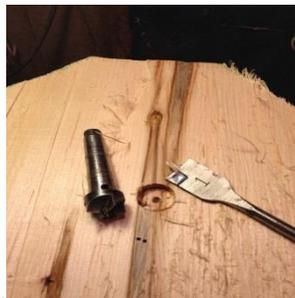
midpoint down the pith line for the drive center. I use a 1" spade bit to make a shallow (1/4") hole for my 1" drive spur. This gives a wall that helps keep the spur in place should the spur tear loose from the fibers.
