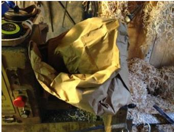
air. Air temperature and humidity are also factor. **CAUTION:** Once you commit to starting the drying process **DO NOT** try turn it any more. It can explode! Cool and humid is best. **NOTE:** after the piece is dry the bottom will not be flat anymore. This will require a re-turn on the lathe to true up the base. For this reason you need to leave a center point for mounting. Then the bottom has a final sanding. Or you can make three feet that will not wobble.
