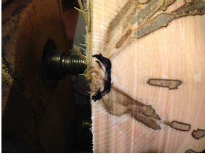
It is important to NOT have the pith in or near the lip of your bowl. Cracks often radiate from the pith and will ruin your work. General rule of 1" below pith or clear of any existing cracks. It is also important to have sharp tools and cut "downhill" or "downgrain".
