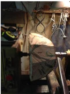
Mount blank on the lathe with the surface vertical and parallel to drive head. You will make some adjustment later. Bring up the tail stock and begin turning. Working from the bottom to top, refine the shape leaving a tenon on the bottom to grab with a chuck.
