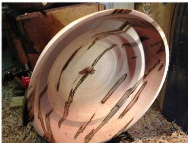
Mount the bowl in your chuck and hollow out the the inside of the bowl, working from the rim down. As a good practice, at about half way down the side, go to the center and establish the final bottom of the bowl. MEASURE TWICE. This will give a point to work toward and not blow through the bottom. Once the inside is finished, you will need to reverse turn the
