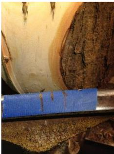
By now the bark should be coming off leaving a "saddle" effect on the sides. Do the same thing with the bottom of the bark lines as with the pith. This will hopefully assure that the two axis of the wood are symmetric, vital in even warping.
