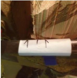
At the point that you get it almost round you need to make an adjustment to the two axis of rotation: PITH axis and BARK axis. This is a most important step in the symmetry process. Put a piece of tape on the tool rest and mark where the each pith passes. If there is any difference in the two marks hold the block steady, with one pith next to tape and loosen the tail live center and split the difference in the two marks. This should ensure that both piths are in the same plane; symmetry.
