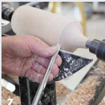
7 Cutting the left side of a cove illustrates the combination of the cutting arcs. Vertically, the tool handle moves upward; laterally, to the left; and rotationally, counterclockwise, with the flute twisting from 3 o'clock to 12 o'clock.
